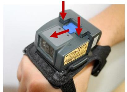
Remove the battery pack from the Tinyom II
